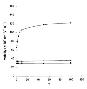
Fig. 2. Mobilities in a capillary filled with the sample buffer as a function of  $\gamma = C_2/C_1$  ( $C_2 = 20$  mM, pH 6.0). ( $\spadesuit$ ) Electroosmotic mobility, ( $\bigcirc$ ) electrophoretic mobility of AsV and ( $\blacksquare$ ) electrophoretic mobility of MMA.
