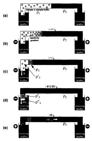
Fig. 1. Schematic representation of the stacking process: (a) hydrodynamic injection of a large sample volume, (b), (c) and (d) backout step, (e) classical separation process after polarity switching.
