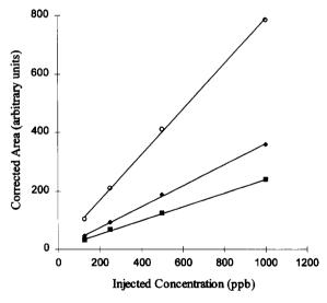
Fig. 4. Calibration curves obtained for MMA ( $\blacksquare$ ), DMA ( $\blacklozenge$ ) and AsV ( $\bigcirc$ ): stacking process for hydrodynamically injected sample volumes corresponding to 50% of the capillary volume. The correlation factors are  $r^2(\text{DMA}) = 0.9992$ ,  $r^2(\text{MMA}) = 0.9992$  and  $r^2(\text{AsV}) = 0.9995$ . Experimental conditions similar to those in Fig. 3.
